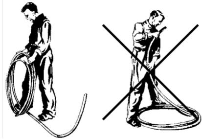
2. Metal hoses must be installed without interference in their natural position and in movement, do not allow the installation to reduce the value specified by the manufacturer minimum bending radius of the metal hose.
